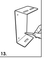
Using wall fixing bracket as template, mark out 4 off drill holes at top and bottom of bracket.
