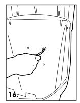
Holding container up to wall bracket, place 4 off M6 x 16mm screws and washers provided through holes on inside of container and fix with nyloc nuts using your fingers. Using a 10mm wrench and allen key provided tighten nuts until secure.
