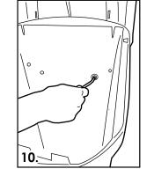
From inside of container, place 4 off screws with washers provided through holes and fix on back of container with washers and nyloc nuts (using your fingers.) Using a 10mm wrench and allen key tighten nuts until secure.
