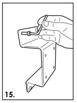
Align wall fixing bracket with drilled holes and screw 4 off M5.5 x 50mm screws provided into wall using security allen key.
