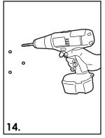
Using a 7mm diameter masonry bit, drill 4 off holes into wall. Place a plastic anchor provided into each drilled hole.
