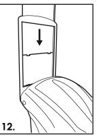
Place graphic behind clear polycarbonate sheet and slide into graphic holder so that lugs locate into slots along bottom of graphic holder.
