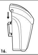
With the 3 off brackets already attached to the container, hook the container onto wall bracket so that the hooks locate into the slots.
