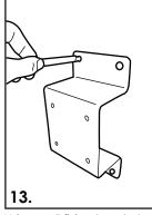
Using wall fixing bracket as template, mark out 4 off drill holes at top and bottom of bracket.
