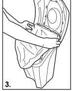
With lid open, install correct size sack (approx 13 " x 21" x 23<sup>1</sup>/<sub>2</sub> " available from Glasdon) by firstly hooking onto retention luas at back of container.
