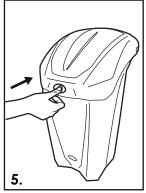
The Confidential Paper model comes complete with push lock located on front of container. With lid closed, push lock centre to lock unit.
