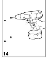
Using a 7mm diameter masonry bit, drill 4 off holes into wall. Place a plastic anchor provided into each drilled hole.
